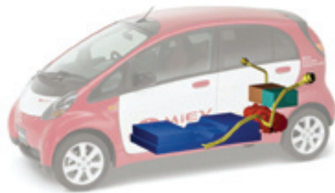
Cut-away illustration showing the internal placement of batteries and charging connectors on Mitsubishi's i-MiEV.
