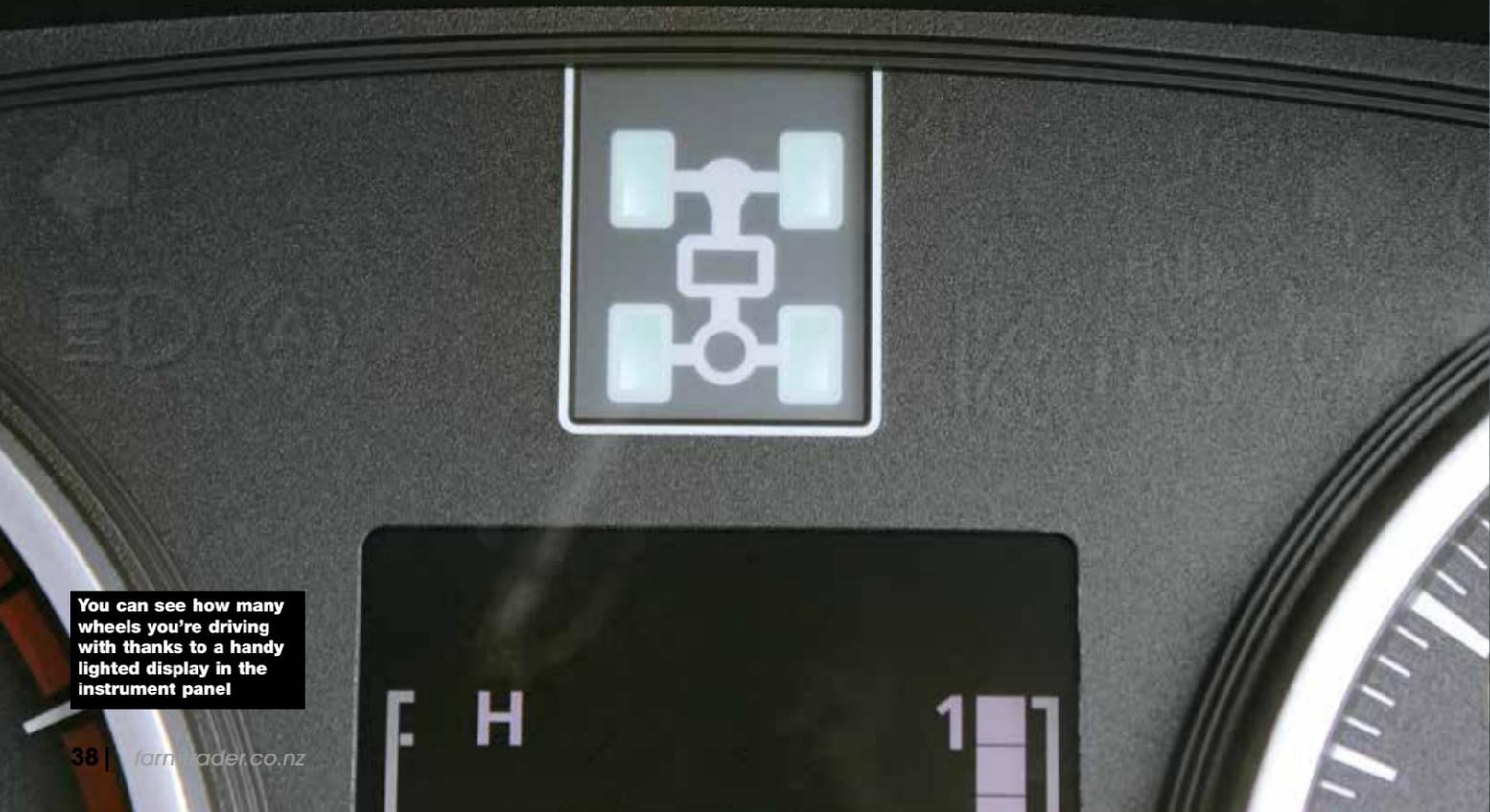
You can see how many wheels you're driving with thanks to a handy lighted display in the instrument panel
