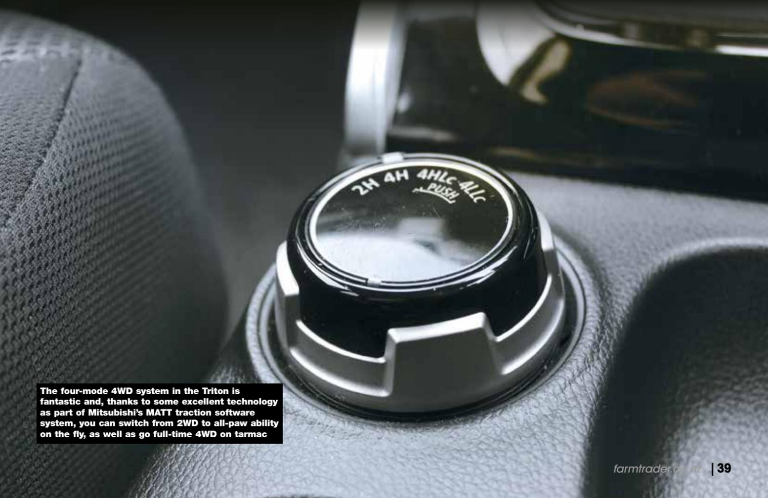
The four-mode 4WD system in the Triton is fantastic and, thanks to some excellent technology as part of Mitsubishi's MATT traction software system, you can switch from 2WD to all-paw ability on the fly, as well as go full-time 4WD on tarmac
