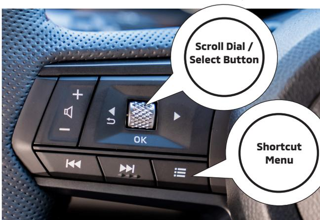
The multi-information display shows warning and information critical to the vehicle. The display can be changed using the ◀ and ▶ buttons and scroll dial located on the steering wheel.
