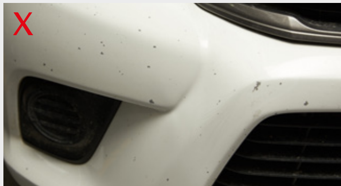
Excessive stone chipping
