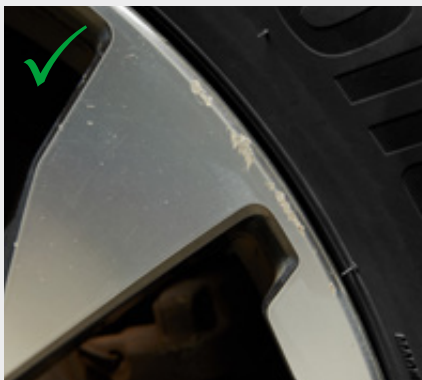
Minor scuff to wheel
