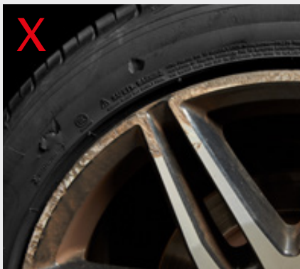
Excessive Damage to wheels
