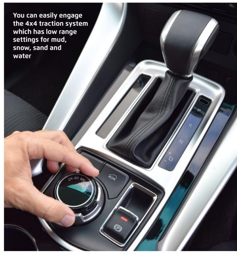
You can easily engage the 4x4 traction system which has low range settings for mud, snow, sand and water
